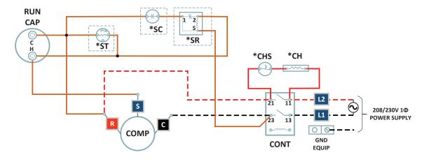
Fig. 2 Installing SmoothStarter
