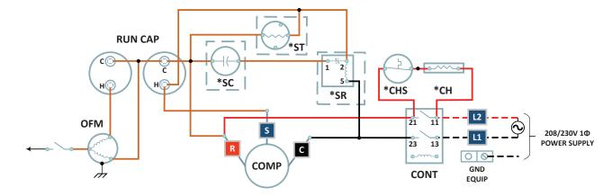
Fig. 2 Installing SmoothStarter
