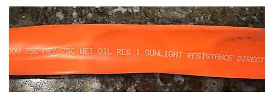
In summary, there may be confusion when the cable's temperature rating differs from the temperature associated with an "Oil Resistant" rating for the cable and/or cable fitting. To avoid any confusion, the following guidelines are provided. The temperature ratings of the cable determine ampacity and should not be correlated with the temperature associated with an "Oil Resistant" rating for the cable and/or cable fitting.
